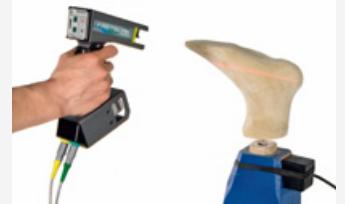
Fig. 12 Scanning a positive shoe last (manufacturer: Spenle).
